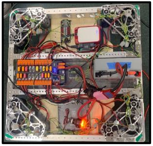
This is the completed drivetrain. This year the team has successfully built and programmed a swerve drive. With just a few adjustments being made, it will be ready for gameplay! This is the official intake prototype, made as an over the bumper solution. The horizontal rollers on the intake compress the game pieces and can grab cones and cubes from anywhere on the ground.
