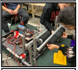
In this photo the team is prototyping the intake. The goal of the intake is to put the cones and cubes into the indexer. The indexer makes sure the cones and cubes are in the right position, so that they can be placed to score points.
