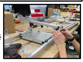
The students are making some final adjustments to the elevator. The code for the elevator is complete, and all that is left is to manufacture the remaining pieces and to piece it together.
